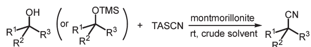
Scheme 1. Direct Transformation of Alcohols or their TMS Ethers with Trialkylsilyl Cyanide (TASCN) to Nitriles
